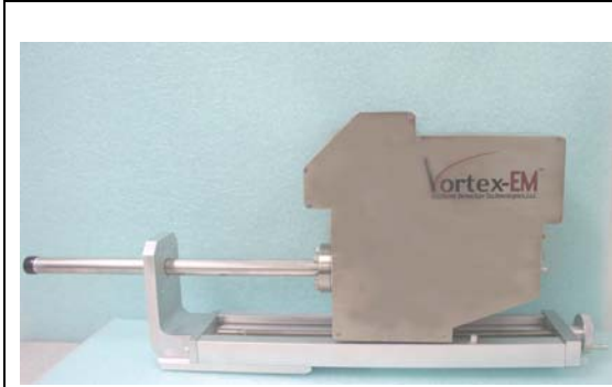
Figure 1. Photograph of the spectrometer designed for the JEOL 840 SEM. Probe length is 12”.
